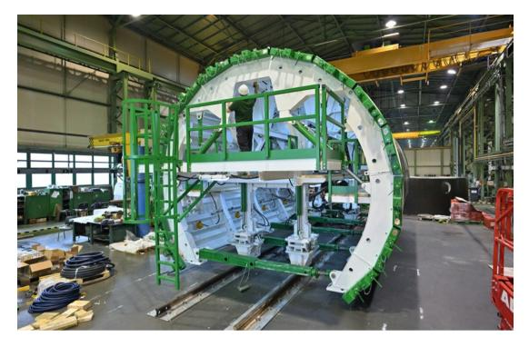
We are a key supplier of formwork equipment for the concreting of the D line of the Prague metro. Our mobile steel formwork is also used in Norway, where it is used as a secondary lining of excavated road tunnels.
